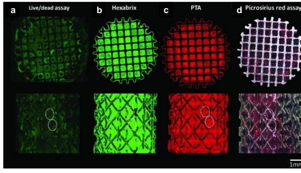
Imaging cell and matrix formation inside a titanium scaffold; a: live/dead assay; b,c: contrast enhance nanoCT; d: picrosirius red assay
