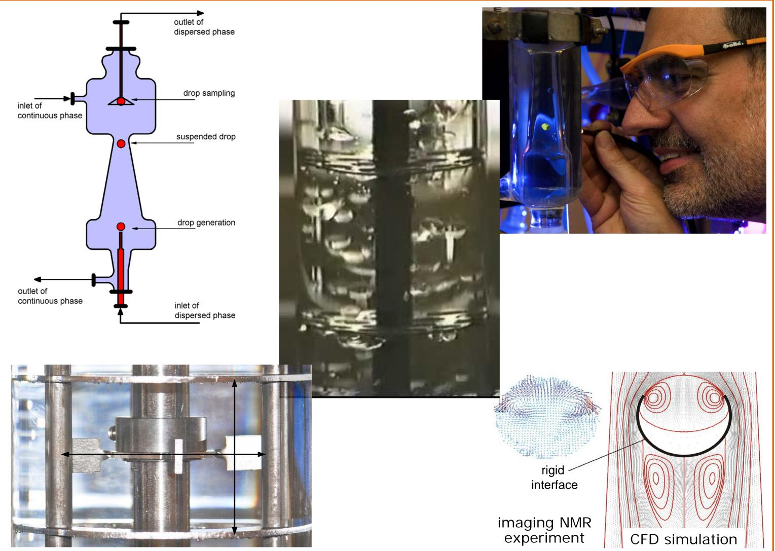
The advantage of **drop-based modelling** is the ability to extrapolate beyond the region of data acquisition, e.g. for **all types of column internals** without any additional experiments. Our **ReDrop program (representative drops)** depicts extraction-column performance including reactions in either phase as well as reactive extraction, where the reaction occurs at the interface, with **better than 10% accuracy**.
