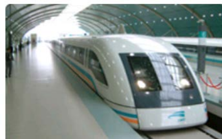
Strong magnets for MAGLEV magnetic levitation train (magnets of several teslas!)
