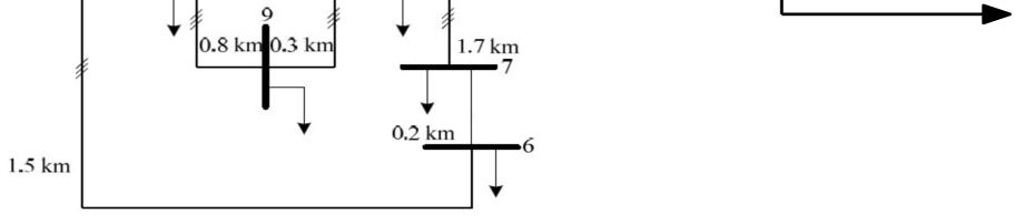
The outputs of interest are the active (P(t)) and reactive (Q(t)) powers entering the distribution grid. Applied voltage dip :  $\Delta V = 0.5$  pu,  $\Delta T = 0.25$  s
