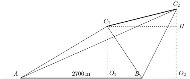
$$\text{tg } \widehat{C_1C_2H} = \frac{\overline{C_2H}}{\overline{C_1H}} = \frac{\overline{C_2O_2} - \overline{C_1O_1}}{\overline{AO_2} - \overline{AO_1}} \rightarrow \widehat{C_1C_2H} = 20^\circ.$$
